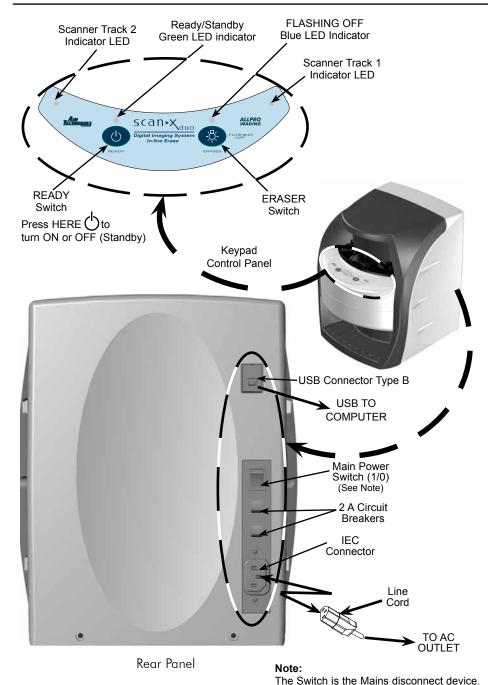
Figure 4. Typical ScanX Duo Installation
