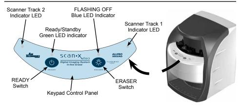
Figure 2. ScanX Duo Front Panel Controls and Indicators
